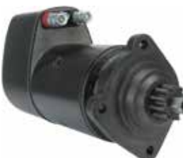
110535 Starter 24 V, 5.4 kW Replacing: 19024035 Servicing: Fiat, Iveco B- M10, B+ M10, Length 384.00, Drive type Steel, Gear type DD, Mount. holes 3 (0) A: 89.00 B: 47.00 mm
