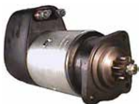
110533 Starter 24 V, 5.4 kW Replacing: 19024011 Servicing: Steyr B- M10, B+ M10, Length 387.00, Drive type Steel, Gear type DD, Mount. holes 3 (0) A: 89.00 B: 46.50 mm
