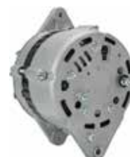
110458 Alternator 14 V, 60 Amp Replacing: LR160-44, LR160-82, LR160-82B, LR160-84, LR160-84B Servicing: Nissan Terminal W, Pulley P, Grooves 1, B+ M5, Length 177.60 A: 43.00 B: 13.00 C: 80.00 mm
