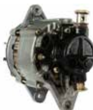
110567 Alternator 28 V, 25 Amp Replacing: LR225-403, LR225-60, LR225-65, LR225-65B, LR225-65C, LR225-65E, LR225-65P, LR225-67, LR225-67B Servicing: Nissan Pulley DP, Grooves 2, B+ M6, Length 248.00 A: 42.10 B: 13.60 C: 81.10 mm
