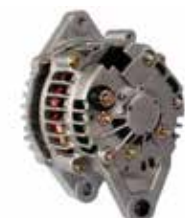
110631 Alternator 14 V, 70 Amp Replacing: LR165-708, LR165-708B, LR165-708C, LR165-708E, LR170-738, LR170-738B, LR170-738C, LR170-738E Servicing: Nissan Pulley SP, Grooves 4, Fan IF, B+ M6, Length 160.00 A: 38.00 B: 24.85 C: 82.20 mm
