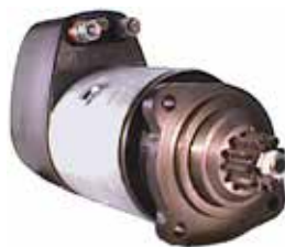
110534 Starter 24 V, 5.4 kW Replacing: 19024030 Servicing: Ford, Iveco, Various Agriculture Vehicles B+ M10, Length 390.00, Drive type Steel, Gear type DD, Mount. holes 3 (0) A: 89.00 B: 47.00 mm
