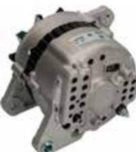
110134 Alternator 14 V, 55 Amp Replacing: LR150-165 Servicing: Mazda Pulley P, Grooves 1, B+ M5, Length 171.50 A: 41.00 B: 12.50 C: 80.50 mm
