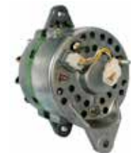
110128 Alternator 14 V, 35 Amp Replacing: LT125-06, LT125-06B, LT125-65, LT130-72, LT130-72B, LT130-75, LT130-81, LT130-83, LT133-03 Servicing: Nissan, Chevrolet, Subaru, Komatsu, TCM Pulley P, Grooves 1, Fan EF, B+ M5, Length 161.00 A: 42.00 B: 13.00 C: 80.50 mm
