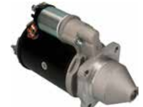
110565 Starter 12 V, 2.8 kW Replacing: 19024817 Servicing: Eicher, Massey Ferguson B- M8, B+ M8, Length 313.00, Drive type Steel, Gear type DD, Mount. holes 3 (0) 4 KW: HC-CARGO 115392. A: 89.00 B: 29.50 mm
