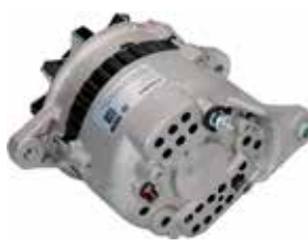
110264 Alternator 14 V, 40 Amp Replacing: LR135-107, LR135-108, LR135-132, LR135-133, LR135-61, LR135-61B, LR135-70, LR135-70B, LR138-01 Servicing: Nissan Pulley P, Grooves 1, B+ M5, Length 159.00 A: 41.50 B: 13.20 C: 80.20 mm
