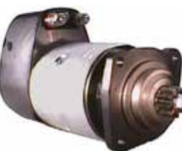
110537 Starter 12 V, 3.6 kW Replacing: 19024000, 19024561, 19024562 Servicing: Mercedes-Benz, Volvo BM B- M10, B+ M10, Length 384.50, Drive type Steel, Gear type DD, Mount. holes 3 (0) A: 89.00 B: 48.00 mm
