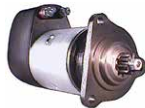
110539 Starter 12 V, 3.6 kW Replacing: 19024008 Servicing: Claas, Mercedes-Benz, New Hol- land B- M10, B+ M10, Length 384.50, Drive type Steel, Gear type DD, Mount. holes 3 (0) A: 92.00 B: 47.00 mm
