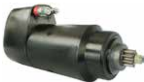
110531 Starter 24 V, 6.6 kW Replacing: 19024071 Servicing: Fiat-Allis, Gmeinder, KHD, Mercedes-Benz B- M10, B+ M12, Length 405.00, Drive type Steel, Gear type DD, Mount. holes 0 (0) A: 56.00 B: 37.00 mm
