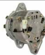
110448 Alternator 28 V, 20 Amp Replacing: LR220-23, LR220-24 Servicing: Mitsubishi, Various Agriculture Vehicles Terminal W, Pulley P, Grooves 1, B+ M5, Length 165.00 A: 44.50 B: 13.50 C: 81.30 mm
