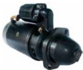
110530 Starter 12 V, 3.0 kW Replacing: 19024238 Servicing: Huerlimann, Lamborghini, Same B+ M10, Length 342.00, Drive type Steel, Gear type DD, Mount. holes 2 (0) A: 82.50 B: 22.00 mm
