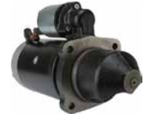
110551 Starter 12 V, 3.0 kW Replacing: 19024815 Servicing: Lamborghini, Same, Ursus, Zetor B+ M10, Length 326.50, Drive type Steel, Gear type DD, Mount. holes 3 (0) A: 89.00 B: 47.00 mm
