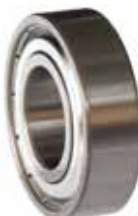
140285 FAG 6003-2Z Replacing: 1900905123 ID 17.00, OD 35.00, Height 10.00 Alternative no.: 142286 CAR GO High Performance
