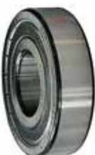
140293 FAG 6306-2Z Replacing: 1900905330 Servicing: 0120600007 ID 30.00, OD 72.00, Height 19.00
