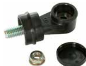
138629 Terminal Kit Replacng: A450X20771 Servicng: A002T35791, A002T35791A, A004T01693, A2T35791, A2T35791A, A2T35792A, A3T09591, A4T01693, A4T02691 Total length 55.00, Thread size M8 B+.
