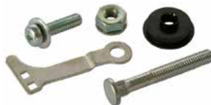
137843 Terminal Kit Replacng: A450X16871, A450X20871, MD611431, MD611483 Servicng: A002T02271, A002T02471, A002T02671, A002T02771, A002T02871, A002T02977, A002T03171, A002T06871 Total length 46.50, Thread length 28.50, Thread size M6
