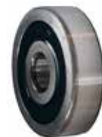
140878 FAG 6403-2RS1 Servicing: 0120468135, 0120468144, 6033GB3021 ID 17.00, OD 62.00, Height 17.00
