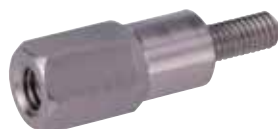
139216 Adaptor Servicing: A127, 63320317, 63321434, 63341434, 63320309, 63320310, 63320315, 63321243, 63321285, 63321346, 63321358 Total length 34.60, Thread length 11.00, Thread size M5/M6
