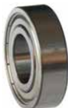
140284 FAG 6002-2Z Replacing: 1900905122 ID 15.00, OD 32.00, Height 9.00
