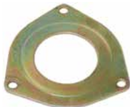
234714# Bearing Plate Servicing: A127I, 063321940010, 063377005010, 63321507, 63320333, 63321232, 63321241, 63321245, 63321246, 63321310 ID 30.00, OD 61.00, Thickness 2.50, Width 50.80, No./mount. holes 3, Material Steel
