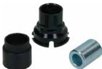
330311 B+ Insulator Servicng: A002TJ0291, A002TJ0291ZE, A003TJ2481, A003TJ2481ZE, A2TJ0281ZE, A2TJ0291, A2TJ0291ZC, A2TJ0291ZE ID 14.50, OD 24.50, Height 24.50
