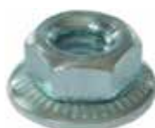
B191306 Hex Flange Nut Replacing: 85-2201 Servicing: 0002801V003, 0002801V004, 0003250V007, 0071549202, 0071549902, 0091549902, 0101540002, 0101548902 Thread M4, Spanner size 7, Coating Electro galvanized, Material Steel Alternative no.: 191306
