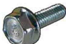
B191327 Hex Flange Screw Replacing: ARS1001, S-3915 Servicing: 0001501750, 0121715001, 0124525074, 0124525093, 0124525527, 03C903023A, 0986030760, 0K01218300 Thread M4, Spanner size 7.00, Length 12.00, Coating Electro galvanized, Material Steel, DIN norm 6921 Alternative no.: 191327
