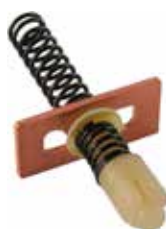
237893 Moving Contact Servicing: 428000-0720, 428000-1620 OD 2 8.20, Length 24.50, Thickness 1.60, Width 26.50, Material Copper, Shaft w/
