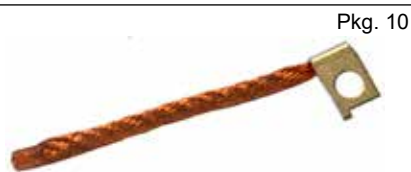
230793 Terminal Lead ID 8.50, Length 23.20, Lead length 106.80, Width 14.30, M8.
