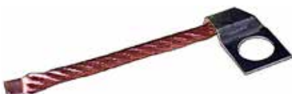
134921 Terminal Lead ID 10.35, Length 26.35, Lead length 68.20, Width 14.65 M10.
