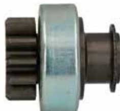
335621 Drive Replacing: 36160-4X902 Servicing: 03111-4300 ID 12.00, OD 37.00, OD/housing 48.50, Total length 50.60, Splines A 10, No./teeth 12, Drive type Steel, Rotation CW
