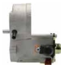
235473 Solenoid Assy Servicing: 03111-4140 12 Volt, 2.2 kW, B+ M8, OD 81.80, Total length 123.00, No./mount. holes 2, Fork lever w/o
