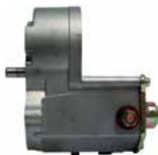
236596 Solenoid Assy Servicing: 03101-3170 12 Volt, B+ M8, ID/cover 75.00, Total length 123.00, Height/B+ 13.50, Terminal 50 6.30, Coil bolt M8, Coil bolt 2 8.50, No./mount. holes 2, No./terminals 3
