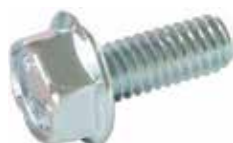
B191326 Hex Flange Screw Replacing: 85-1204 Servicing: 0001106014, 0001106019, 0001106023, 0001107076, 0001107080, 0001107091, 0001107097, 0001107406 Thread M4, Spanner size 7.00, Length 10.00, Coating Electro galvanized, Material Steel, DIN norm 6921 Alternative no.: 191326
