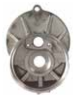
231988 I.M. Bracket Replacing: M640B26571 Servicing: M002T54671, M002T56471, M002T56472, M002T57371, M002T65271, M002T65272, M003T64172, M2T54671 ID 85.00, ID/bearing 32.00, OD 95.50, Height 27.00, Edge height 14.70
