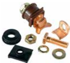
230744 Contact Kit Replacing: 028099-2520, 028099-6390, 028099-6400, 028099-6401, 028099-6410, 028099-6411, 028099-6420 Servicing: 128000-5731, 128000-5732, 228000-7902, 428000-0190, 428000-2370 Shaft dim. M12 24 V. 5.5 kW.
