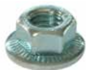
B191307 Hex Flange Nut Servicing: 0001109048, 0001147400, 0001147404, 0002801V003, 0002801V004, 0003250V007, 0003250V008, 0071549202 Thread M5, Spanner size 8, Coating Electro galvanized, Material Steel Alternative no.: 191307
