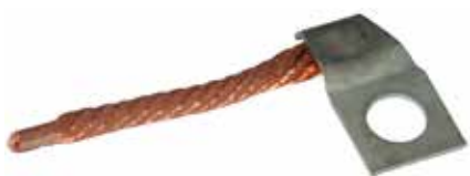
133506 Terminal Lead ID 8.50, Length 26.55, Lead length 52.65, Width 14.65 M8.
