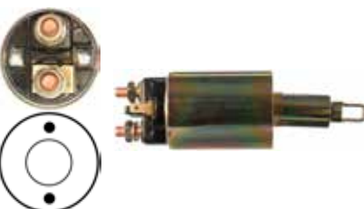
132470 Solenoid Replacing: M371X11171, M371X12571, M371X14571, M371X41971 Servicing: M5T20171, M5T23272, M5T20171, M5T23271 12 Volt, B+ M8, ID/cover 21.20, ID/eye 7.00, OD 52.00, OD/cover 45.35, Length 68.00, Total length 134.20, Height/B+ 14.75, Terminal 50 9.40, Coil bolt M8, Coil bolt 2 15.00, No./mount. holes 2, No./terminals 3, Fork lever w/
