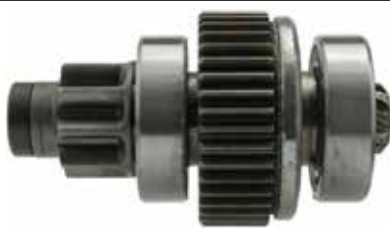
236607 Drive Servicing: 03101-3170, 03101-3190, 03101-3220 OD 29.00, Total length 93.50, Splines A 10, No./teeth 9, Rotation CW, Key spline w/o, Lock w/o
