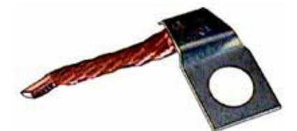
133505 Terminal Lead ID 8.40, Length 26.45, Lead length 39.50, Width 14.75 M8.
