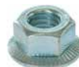
B191513 Hex Flange Nut Replacing: F00M990127, F00M990181 Servicing: 0001106014, 0001106018, 0001106019, 0001106023, 0001107076, 0001107080, 0001107088, 0001107091 Thread M8, Spanner size 13, Coating Electro galvanized, Material Steel Alternative no.: 191513
