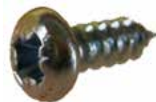
190360 Tapping Screw Replacing: 190333 Dim. 3.5x9.5, Head type Pan head, Material Electro galvanized, Type no. 6, DIN norm 7981C, ISO norm 7049
