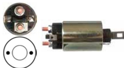
132472 Solenoid Replacing: M371X45971, M372X00171, M372X02171, M372X02371, M372X06871, MD607448, ME700115 Servicing: M002T54272, M002T54871, M002T54881, M002T56471, M002T56475, M002T60185, M003T61071, M003T61171 12 Volt, B+ M8, ID/eye 6.70, OD 55.00, OD/cover 49.10, Total length 148.75, Height/B+ 18.00, Terminal 50 9.40, Coil bolt M8, Coil bolt 2 18.20, No./mount. holes 2, No./terminals 3, Fork lever w/ Cap: HC-CARGO 133286.
