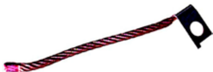
133371 Terminal Lead Servicing: M8 ID 8.45, Length 23.15, Lead length 106.45, Width 14.10
