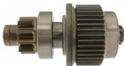
235095 Drive Servicing: 03111-4140, 03111-4240, 03111-4241 ID 9.00, OD 32.00, OD/housing 42.00, Total length 104.00, Splines A 10, No./teeth 10, Drive type Steel, Rotation CW
