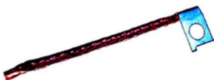
133372 Terminal Lead ID 8.45, Length 23.40, Lead length 106.75, Width 14.10 M8.
