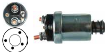
133178 Solenoid Replacing: 35640175 12 Volt, B+ M8, OD 46.30, OD/cover 51.15, Total length 122.00, Height/B+ 19.60, Terminal 50 M5, Coil bolt M8, Coil bolt 2 9.00, No./mount. holes 4, No./terminals 3 Cap: HC-CARGO 131323.
