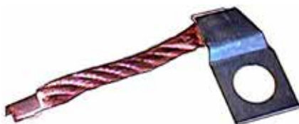
134064 Terminal Lead ID 8.40, Length 26.30, Lead length 53.00, Width 14.65 M8.
