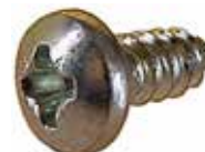
190366 Tapping Screw Replacing: 190339 Dim. 4.2x9.5, Head type Pan head, Material Electro galvanized, Type no. 8, DIN norm 7981C, ISO norm 7049
