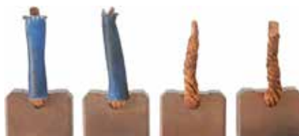
142077 Brush Set Servicing: 03111-4240, 03111-4241 12 Volt, Length 18.05, Lead length 38.00, Lead length 2 38.00, Height 24.85, Thickness 7.80
