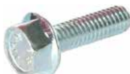
B191328 Hex Flange Screw Servicing: 0002801V003, 0002801V004, 0003250V007, 0003250V008, 04868430AB, 04868430AC, 04868430AD, 04868430AE Thread M4, Spanner size 7.00, Length 14.00, Coating Electro galvanized, Material Steel, DIN norm 6921
