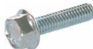
B191329 Hex Flange Screw Replacing: 2910021128 Servicing: 0120300524, 0120400706, 0120400707, 0120400908, 0120400909, 0120489584, 0120489599, 0120489647 Thread M4, Spanner size 7.00, Length 16.00, Total length 20.20, Coating Electro galvanized, Material Steel, DIN norm 6921 Alternative no.: 191329
