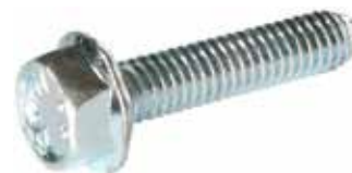
B191330 Hex Flange Screw Servicing: 0051543402, 0061541602, 0071549202, 0071549902, 0091540702, 0091549902, 0101540002, 0101542002 Thread M4, Spanner size 7.00, Length 18.00, Coating Electro galvanized, Material Steel, DIN norm 6921 Alternative no.: 191330
