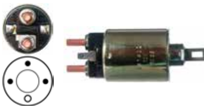
131802 Solenoid Replacing: M371X00272, M371X00382, M371X17271, M371X34471, M371X35071, M371X54471, M371X54671, M371X54771 Servicing: M002T10171, M002T20181, M002T23181, M002T51181, M003T26081, M003T29481, M2T10171, M2T20181 12 Volt, B+ M8, ID/eye 5.25, OD 51.30, OD/cover 44.75, Total length 131.00, Height/B+ 18.25, Terminal 50 6.30, Coil bolt M8, Coil bolt 2 18.25, Fork lever w/, No./mount. holes 4, No./terminals 3 Cap: HC-CARGO 133273.
